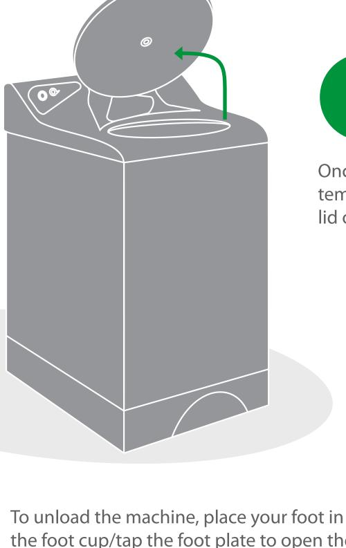
Once the drum has cooled to a safe temperature of 60°C, the machine lid or door can be opened.
