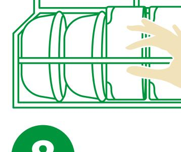
the foot cup/tap the foot plate to open the machine, remove the clean utensils and place on a storage rack to dry.
